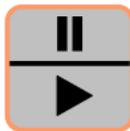
Press this key to stop the measurement. Press again and the measurement will continue.
